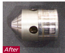
Demag's new Ultra Life™ machine fluid had a "cleaning" effect on Sajar Plastics 500 HP machine as demonstrated by the before and after images (left, top to bottom) of the ejector spool, pump check and the clamp open cartridge.
